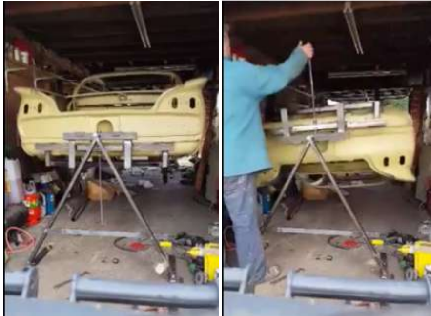
Rotisserie style repairs underway.....
