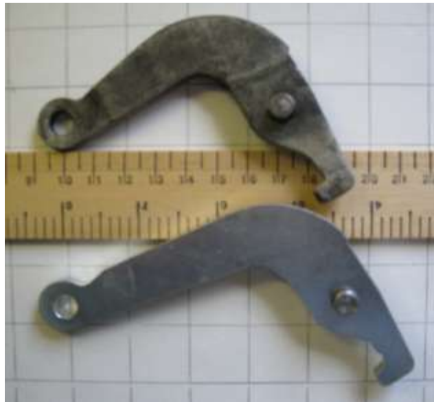
Original and lengthened handbrake levers
