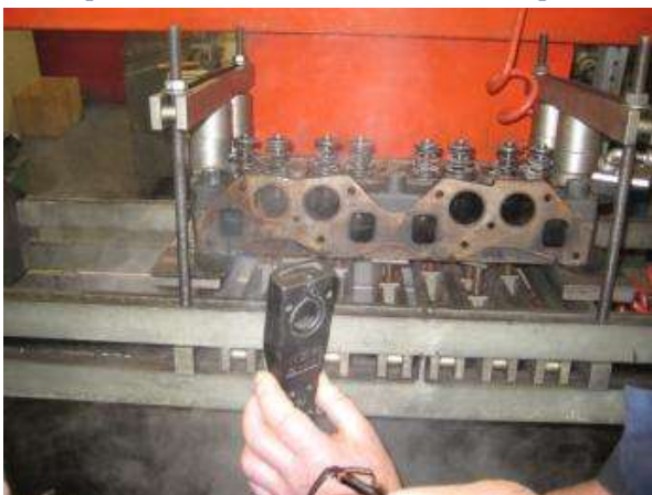
Pressure testing reveals the leak
