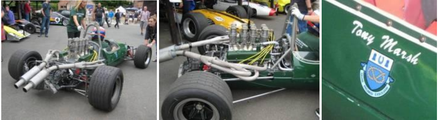
Ex Tony Marsh 4,250 cc 4WD Special, driven here by his sons Simon and Peter
