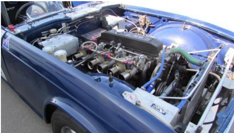
Part of the reason why .....another part.... The horns on the passenger side aren't bass boosters – they are air intakes used to cool the differential...!!!
