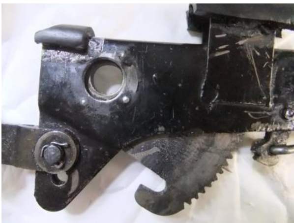
Figure 1 Repositioned compensator link on TR4A handbrake lever
