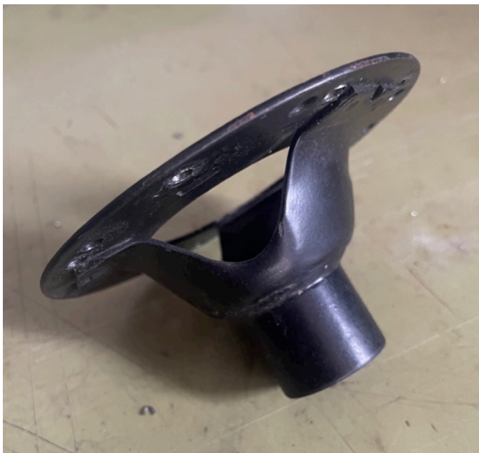
The flimsy looking fabricated Astralli boss is usually covered with a plastic shroud
