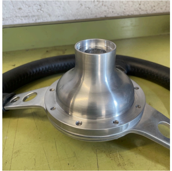
With Helicoils. The machined recess which covers the top of outer column and column top bush can also be seen here.
