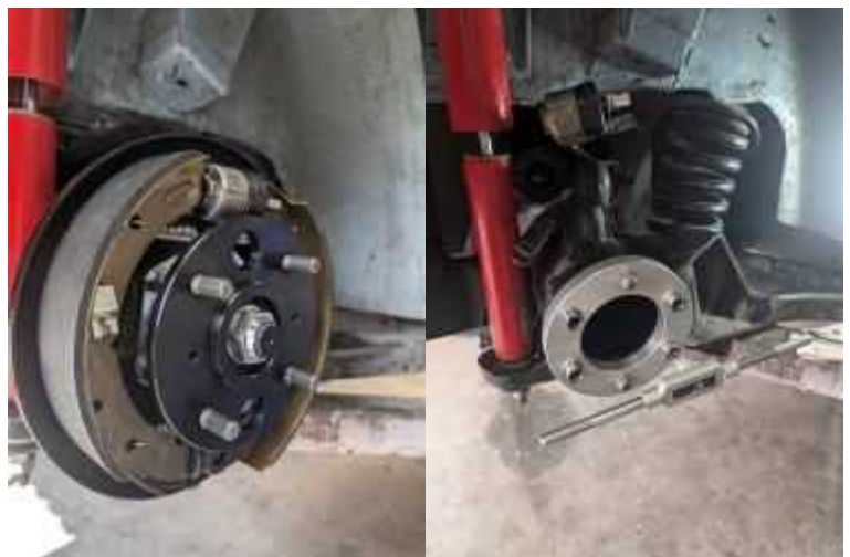
New hub on the left. Template for drilling and tapping larger stud holes on the right.
